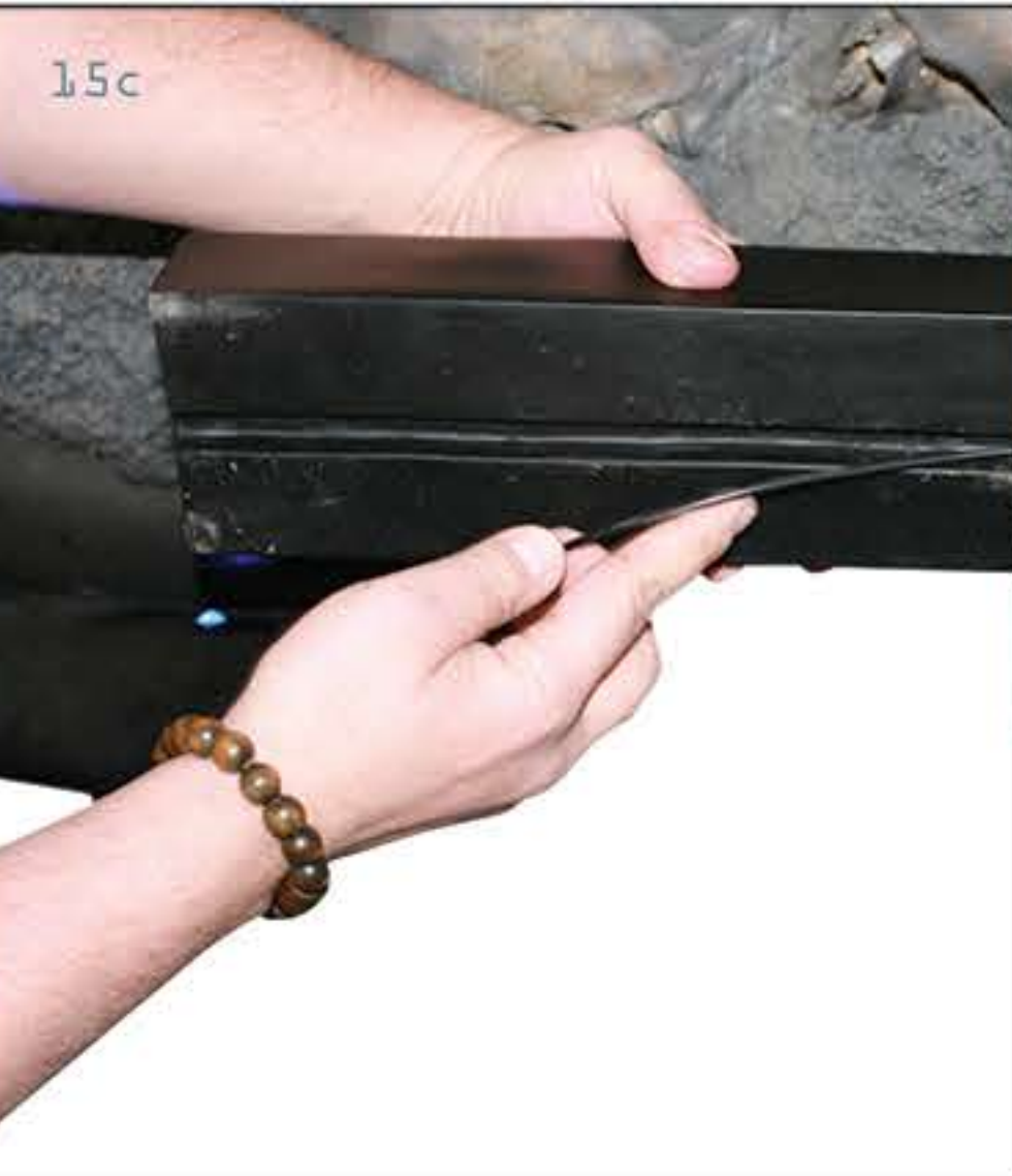
ALIGN POWER CABLE WITH GROOVE IN EXTENSION PIECE. ALIGN EXTENSION PIECES WITH CURVED LIGHTBAR.
