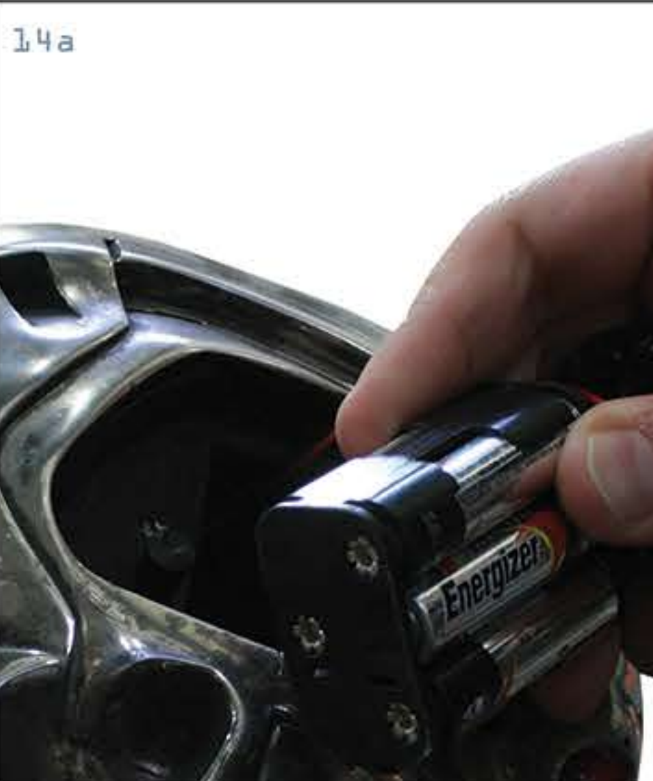
REMOVE COVER PANEL BY PULLING STRAIGHT OUT. PULL BATTERY CARTRIDGE OUT. REPLACE BATTERIES.
