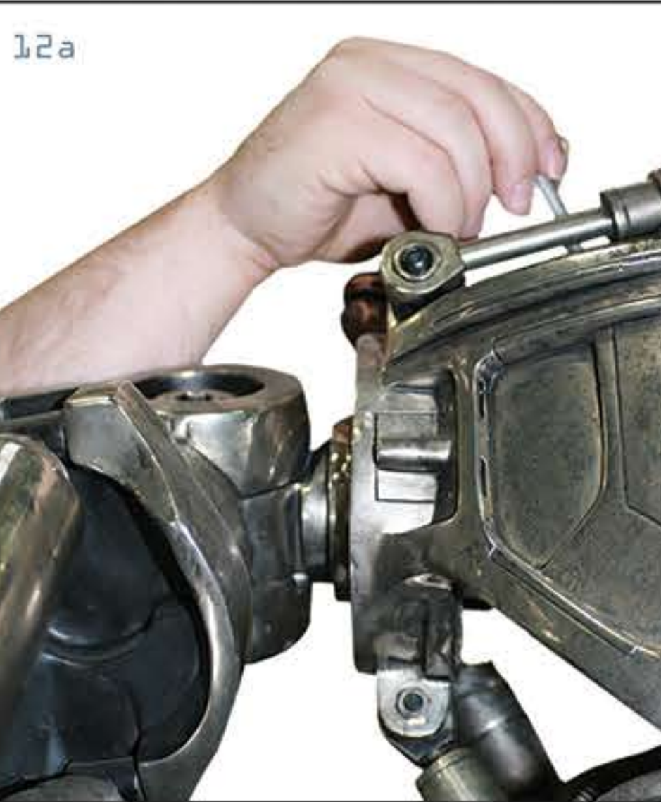
INSERT RETAINING PIN TO LOCK ARM IN POSITION. TO CHANGE ARM POSE, REMOVE THE 'RETAINING PIN.' THEN REMOVE THE ARM. REINSTALL THE ARM AT THE DESIRED POSITION AND INSERT THE RETAINING PIN
