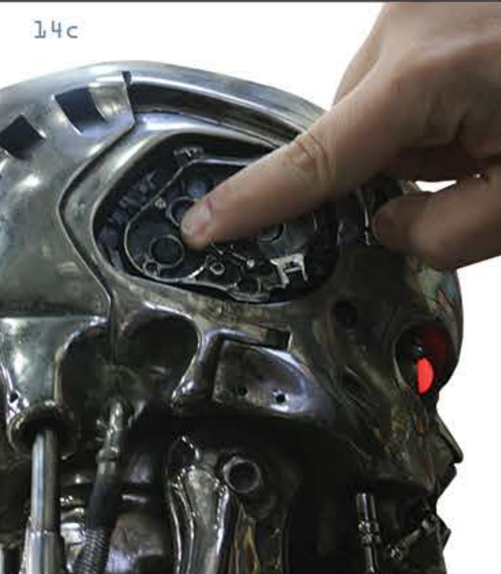
RE-ATTACH BATTERY COVER PANEL BY ALIGNING HOLE WITH POWER SWITCH. PRESS COVER INTO POSITION.
