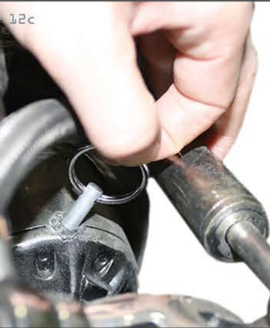
INSERT RETAINING PIN TO LOCK ARM IN POSITION. TO CHANGE ARM POSE, REMOVE THE 'RETAINING PIN.' THEN REMOVE THE ARM. REINSTALL THE ARM AT THE DESIRED POSITION AND INSERT THE RETAINING PIN
