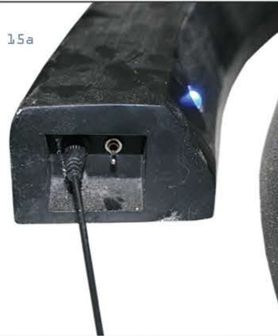
PLUG IN POWER CABLE TO CURVED LIGHTBAR. PLUG POWER CABLE INTO WALL SOCKET. FLIP TOGGLE SWITCH UP FOR STROBE LIGHT. FLIP TOGGLE SWITCH DOWN FOR CONSTANT LIGHT. CENTER TOGGLE SWITCH FOR OFF
